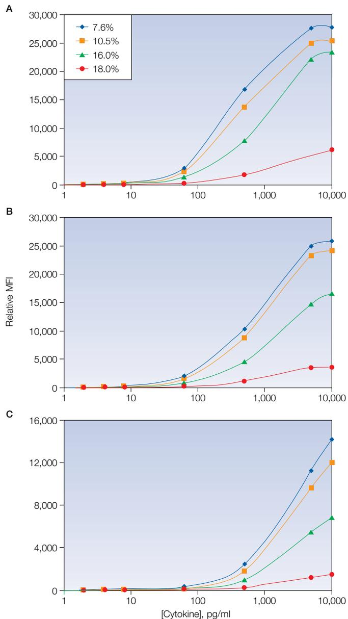
Assays of cytokines on a Bio-Plex system reader with varying degrees of misalignment. A, IL-6 assay; B, IL-8 assay; C, GM-CSF assay. MFI, mean fluorescence intensity.
