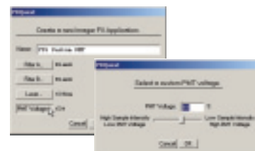
Fig. 2. Fine adjustment of PMT voltage.
