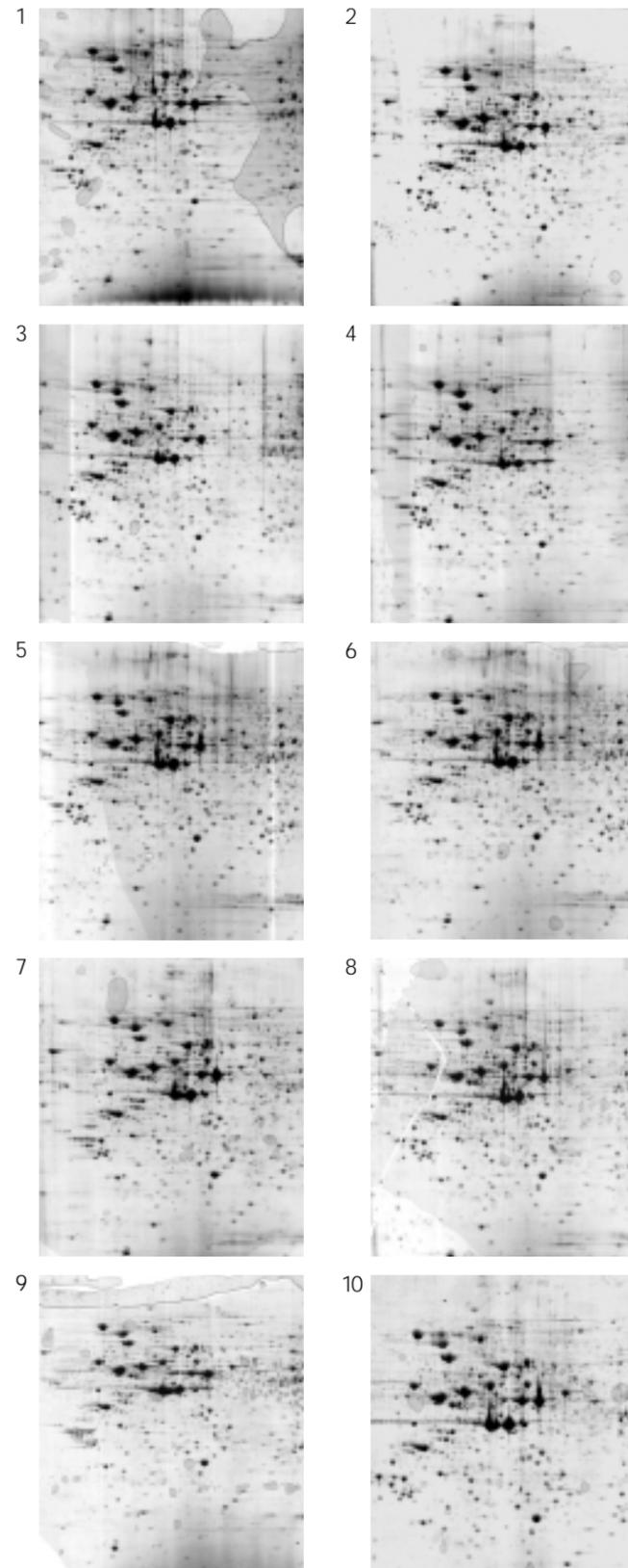
Fig. 2. Images of 10 Coomassie Blue-stained gels run on the Dodeca cell. Gels were 9–16% acrylamide gradients using Laemmli reagents. Proteins (500  $\mu$ g) were loaded from pH 4–7 IPG strips and gels run for 6.5 hr.
