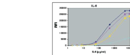
Figure 1. Effect of Misalignment of Optics on Cytokine Standard Curves
