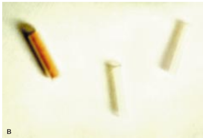
Fig. 1. A. C. elegans worm pellet in the center of an 6 cm Petri dish on ice after microparticle bombardment (conditions are described in detail in Methods). B. Different Au-DNA containing cartridges (16 mm in length) in comparison to each other. The "bullet" on the left border, which shows homogeneous distribution of gold-DNA particles, was prepared by our modified protocol.
