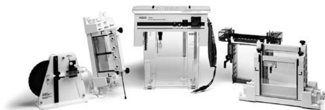
Fig. 1. The DCode system is a flexible system that can be used for any combination of mutation screening techniques. At the center of the system is the temperature control module, which includes a microprocessor-controlled heater, a buffer recirculating pump, and a stirrer. For techniques requiring temperature control, the gels are immersed in the buffer and the temperature is regulated between 5° and 70°C. Temperatures below ambient can be achieved by using the cooling tank in conjunction with an external laboratory chiller.
