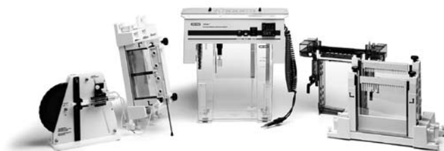
Fig. 1. The DCode system is a flexible system that can be used for any combination of mutation screening techniques. At the center of the system is the temperature control module, which includes a microprocessor-controlled heater, a buffer recirculating pump, and a stirrer. For techniques requiring temperature control, the gels are immersed in the buffer and the temperature is regulated between 5° and 70°C. Temperatures below ambient can be achieved by using the cooling tank in conjunction with an external laboratory chiller.
