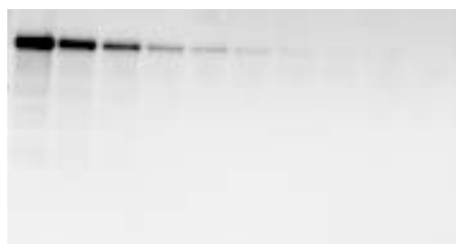
Fig. 1. High signal-to-noise detection using Immun-Blot PVDF membrane. Serially diluted protein transferred to Immun-Blot PVDF membrane was detected using the Immun-Star™ HRP chemiluminescent detection kit and imaged using the VersaDoc™ 3000 system.
