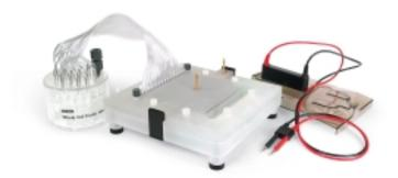
The patented\* whole gel eluter system is available in 14-well (mini whole gel eluter) and 30-well (whole gel eluter) versions with optional collectors and includes consumables for up to 25 runs.
