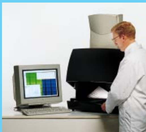
Step 1: Select emission filter(s) and illumination source; Step 2: Position and zoom sample; Step 3: Preview image display; Step 4: Automatically integrate and save the image
