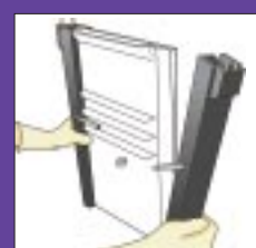
2. Slide and secure full-length lever clamps over gel sandwich.
