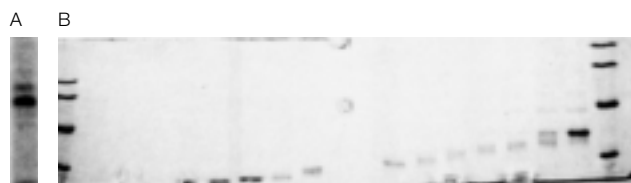
Fig. 1. Separation by preparative SDS gel electrophoresis of a detergent extract of rat adrenal cortex mitochondria. Panel A illustrates the detergent extract prior to treatment on the Model 491 prep cell. Panel B shows two SDS-PAGE gels of fractions obtained after electrophoresis of the crude sample using the Model 491 prep cell. Every fifth fraction after the elution of the dye front from the prep gel was analyzed by removing one-sixth of the fraction and precipitating the protein using TCA. The gels are stained with Coomassie Blue dye. The molecular weight markers seen in the gel on the left and the gel on the right are 97 kD, 66 kD, 43 kD, and 30 kD.
