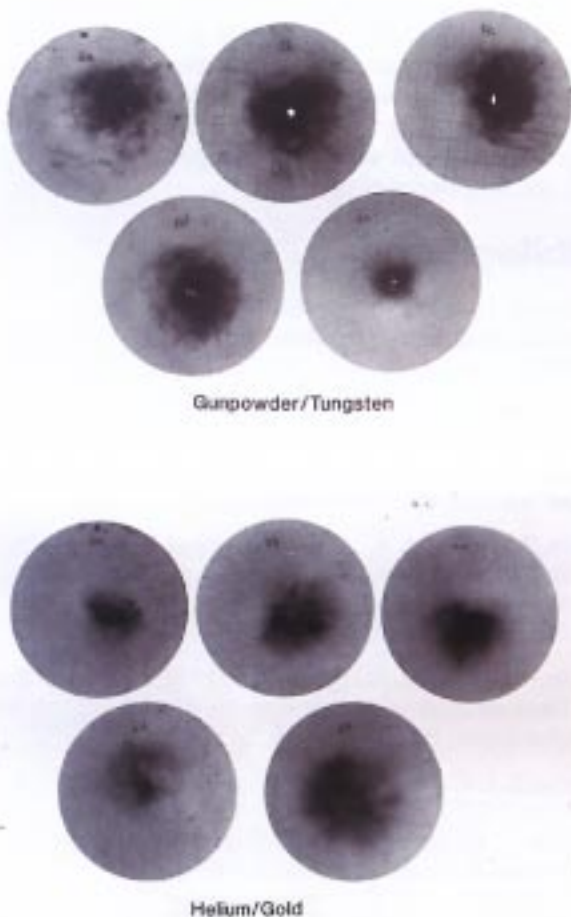
Fig. 8. Particle distribution as revealed by biotin-labeled DNA for the PDS-1000 (A) and PDS-1000/He (B). Membranes were 6 cm from the stopping assembly.
