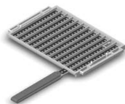
Fig. 2. Removal of ProteinChip arrays from the cassette using array forceps.
