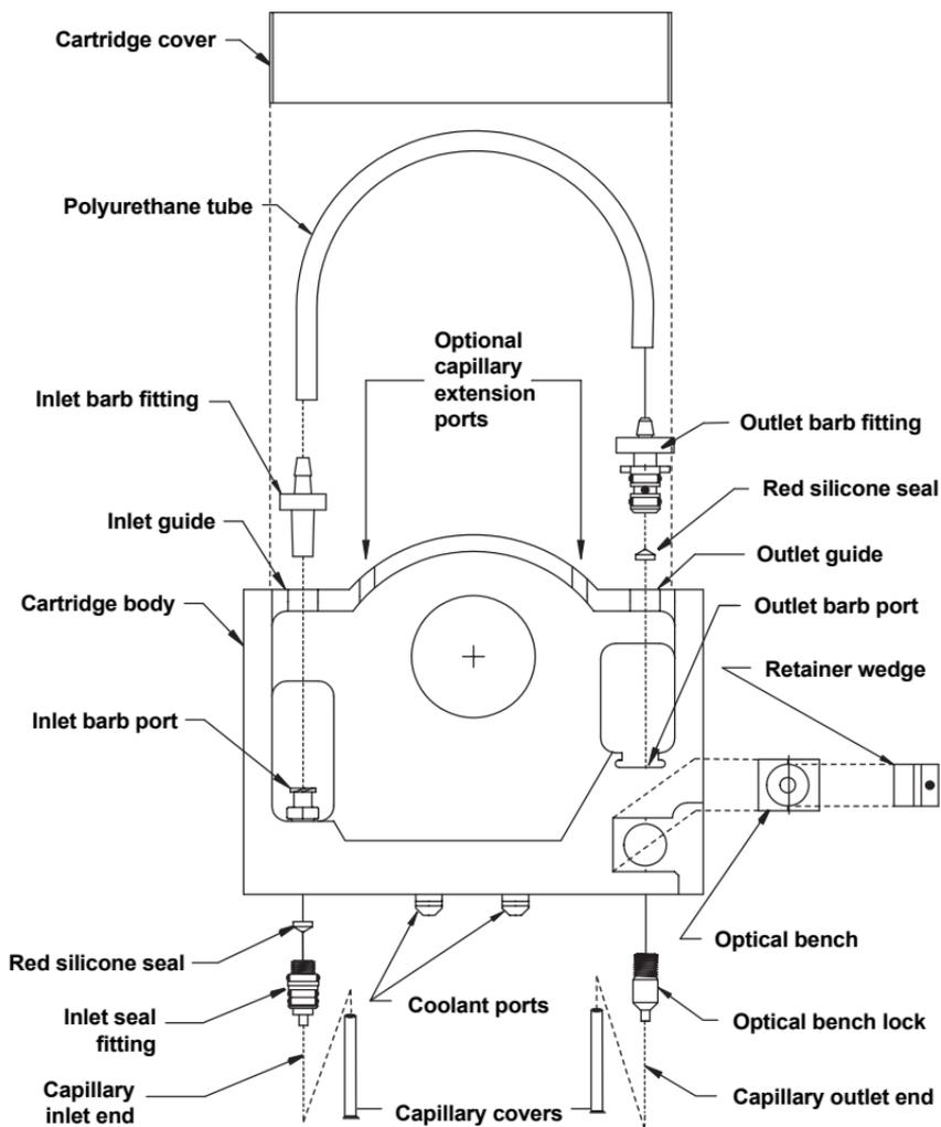
Fig. 1. BioFocus cartridge assembly diagram.
