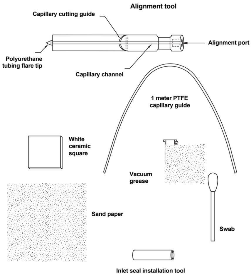
**Fig. 2. Cartridge assembly tools.**
