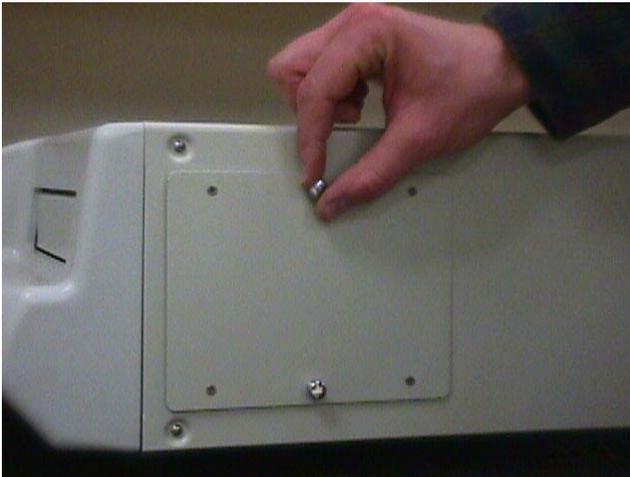
2. Loosen thumbscrews on side panel and remove panel.
