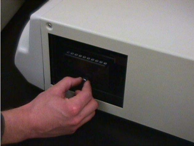
3. Remove thumbscrew holding filter magazine in place.
