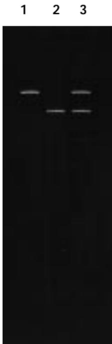
**Fig. 4. Separation of mutant and wild-type DNA electrophoresed on a TTGE gel.** The gel was 8% acrylamide:bis (37.5:1) containing 7 M urea, run at 130 volts for 3 hours in 1.5x TAE buffer, temperature range from 63–66 °C, and ramp rate of 1 °C/hr. Lane 1, mutant DNA, lane 2, wild-type DNA, and lane 3, mutant and wild-type DNA. Excess primers may be seen near the bottom of the gel.
