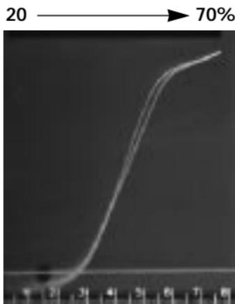
**Fig. 1. Separation of mutant and wild-type DNA electrophoresed on a 20–70% perpendicular denaturing gradient gel.** The gel was 10% acrylamide:bis (37.5:1), run at 130 volts in 1x TAE buffer, heated at 56 °C, for 2 hours.
