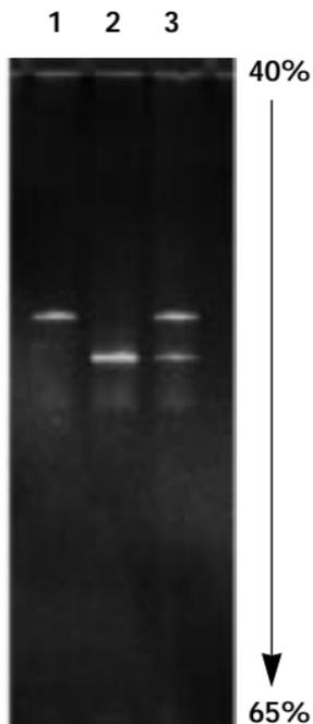
**Fig. 2. Separation of mutant and wild-type DNA electrophoresed on a 40–65% parallel denaturing gradient gel.** The gel was 8% acrylamide:bis (37.5:1), run at 150 volts in 1x TAE buffer, heated at 60 °C, for 2.5 hours. Lane 1, mutant DNA, lane 2, wild-type DNA, and lane 3, mutant and wild-type DNA.
