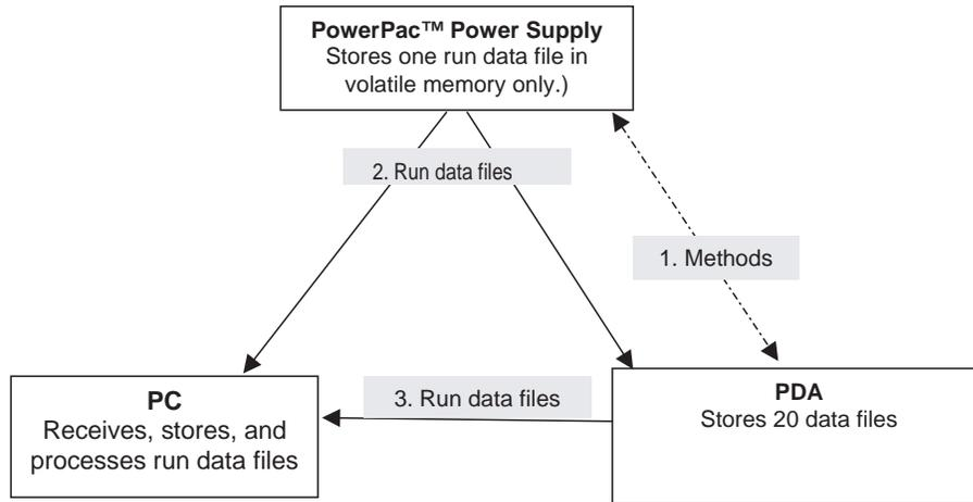
Fig. 3. Data files transfer pathway.
