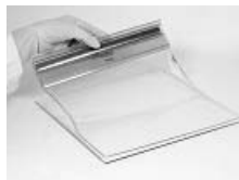
Fig. 2.3.3 B. Clamping onto a PROTEAN Plus precast gel (25.6 X 23 cm).
