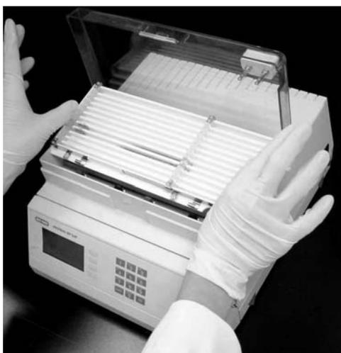
**Figure 10. Removal of Focusing tray from PROTEAN IEF cell.**
