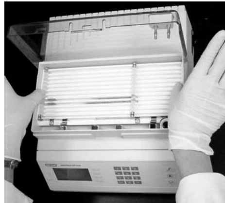
Figure 9. Insertion of Focusing tray into PROTEAN IEF cell.
