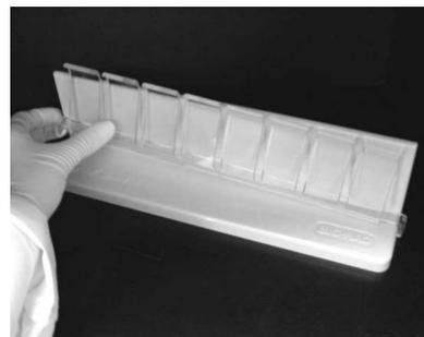
**Fig. 2.1a.** Hook one side of the clamp in the notch.
