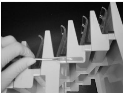
**Fig. 4.2.2a.** Insert a thin spatula under the clamp.
