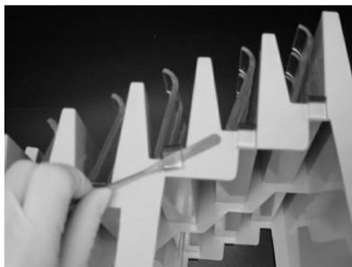
**Fig. 4.2.2b.** Rotate the spatula until the clamp pops off.
