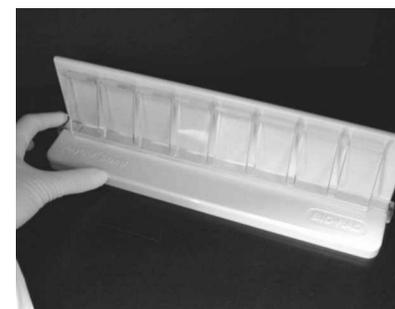
**Fig. 2.1b.** Press firmly to snap on the clamp.
