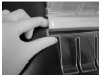
Fig. 2.1c. Snap on the seventh clamp in the front of the 6-row stand.
