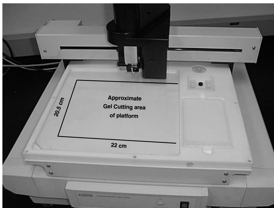
Figure 3. Cutting Platform and Cutting Area.
