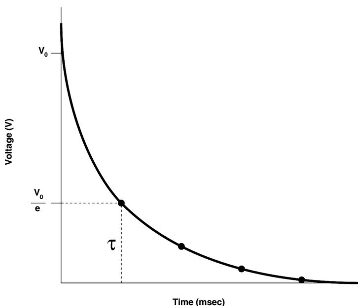
**Fig. 2. Exponential decay pulse from a capacitance discharge system.** When the capacitor, charged to an initial voltage,  $V_0$  is discharged into cells, the voltage applied to the cells decreases over time so that at time  $t = \tau$ , the voltage is  $(1/e) \times V_0$  of the initial value.
