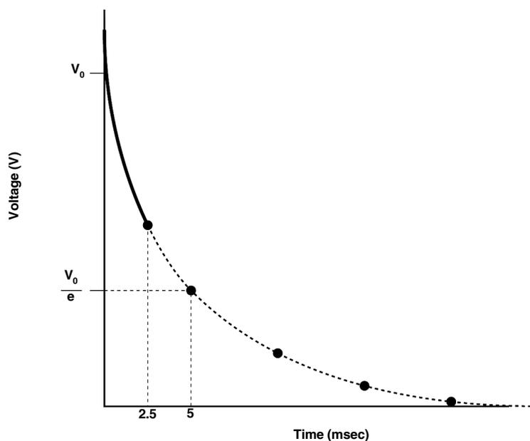
**Fig. 3. Truncation of an exponential decay pulse by the MicroPulser.** The solid line shows the voltage applied to the cells as a function of time during a pulse terminated after 2.5 msec. The dashed line shows the voltage that would normally be applied to the cells during a true exponential decay pulse.
