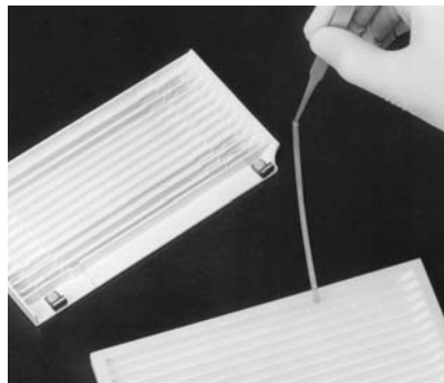
Fig. 3. Draining the oil.
