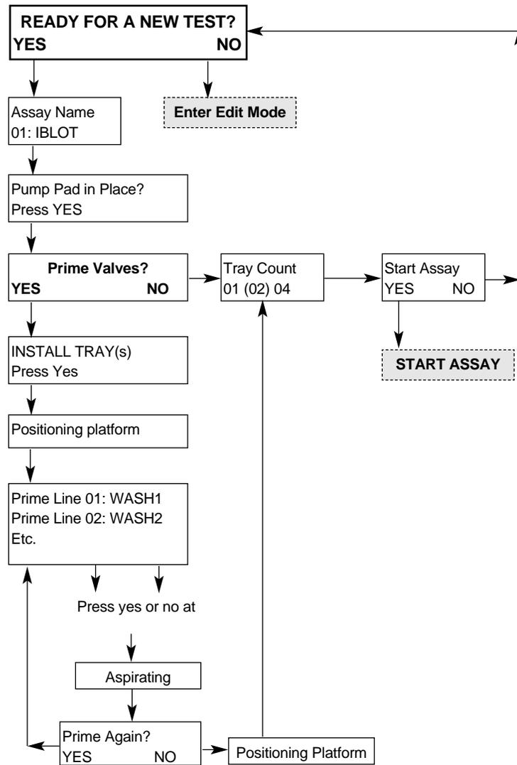
**Note:** When a method is completed, be sure to immediately wash all six (6) lines and valves in the Purge Tubing Mode. If buffer salts and other reagents are allowed to remain in the system, the lifespan of the valves will be greatly reduced.
