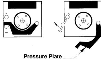
The tension setting on the pump release is preset for optimum performance. Changing the tension of the pump release will adversely affect the calibration and the lifespan of the tubing.
