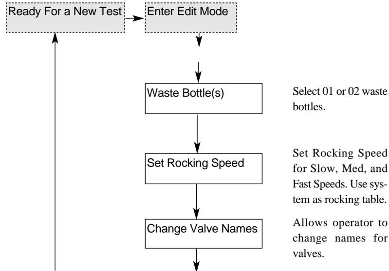
**Note:** The Set Rocking Speed will cycle through FAST, MED, and SLOW speed modes. The preset values for each of these rocking speeds are 30 RPM for FAST speed, 15 RPM for MED speed, and 5 RPM for SLOW speed.
