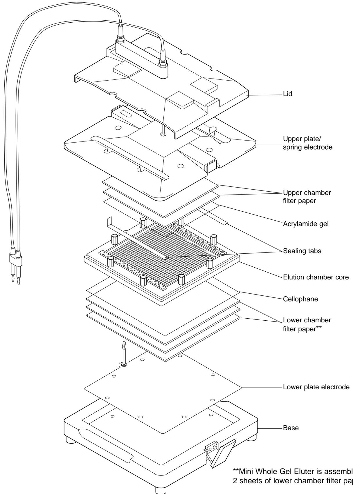
\*\*Mini Whole Gel Eluter is assembled with 2 sheets of lower chamber filter paper.
