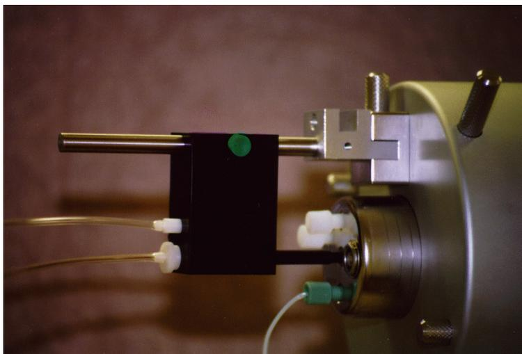
**Figure 8.** Coupling Tee Mounted on Electrospray Interface
