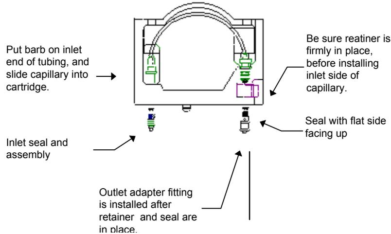
**Figure 5.** Cartridge Assembly
