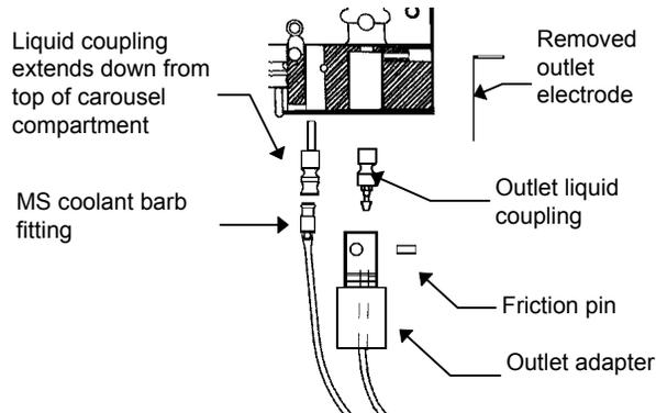
**Figure 6. Installing the Outlet Adapter**
