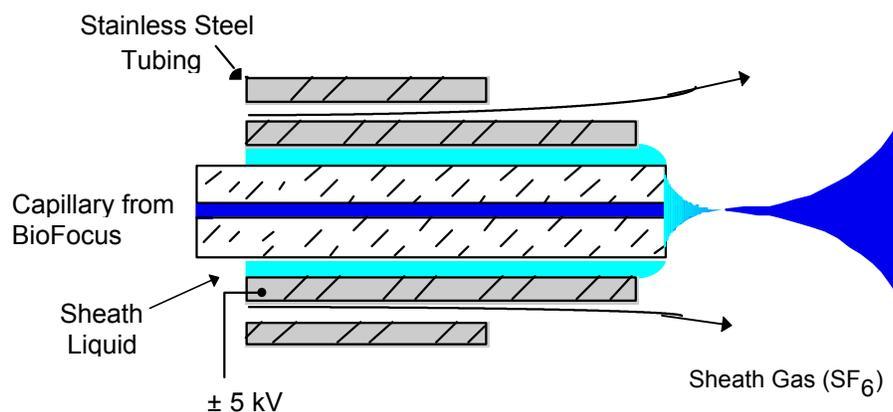
**Figure 1.** Sheath Flow and Sheath Gas Surround Capillary.
