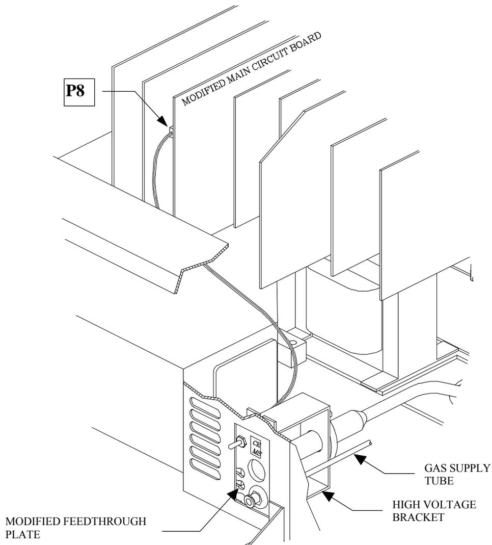
**Figure 2.** Installing the Switch Plate Assembly
