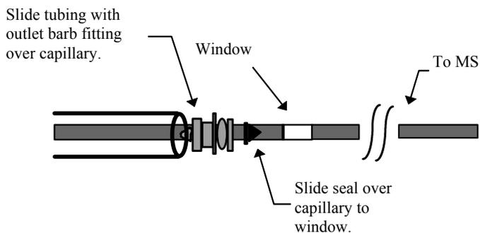
**Figure 4.** Installing the Outlet Seal and Fitting
