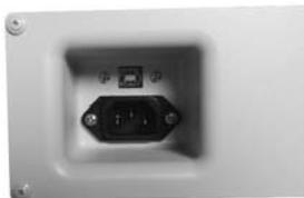
Fig. 3.2. View of USB-2 connection
