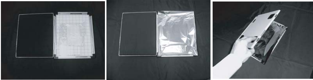
Fig. 4.5. Protective sheet placement steps.
