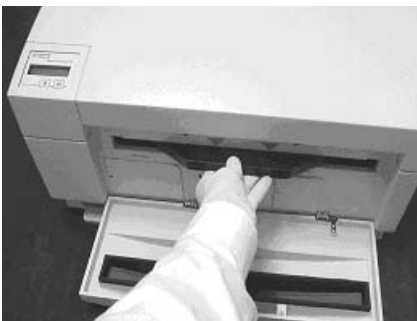
Fig. 4.7. Steps for inserting a screen into the scanner.
