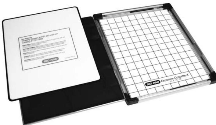
**Fig. 2.2. Sample exposure cassette and phosphor screen.**
