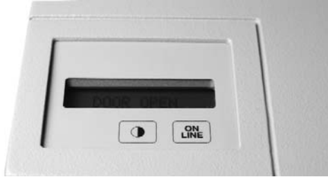
Fig. 4.1. PMI control panel.
