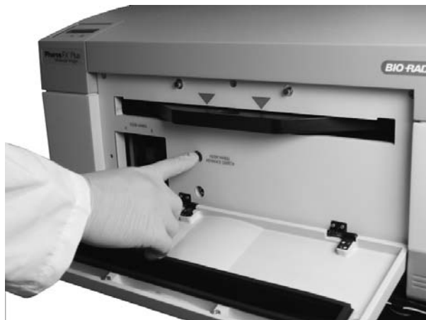
Fig. 4.4. Selecting a filter position using a filter wheel advance switch.
