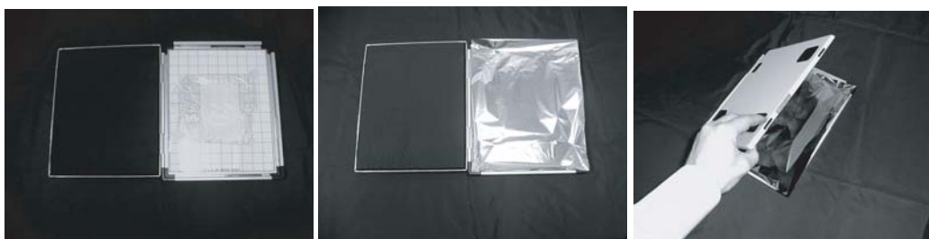
Fig. 11. Use of protective sheet in Imaging Cassette.
