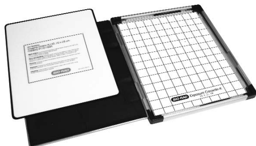
Fig. 2.4. Sample exposure cassette and phosphor screen
