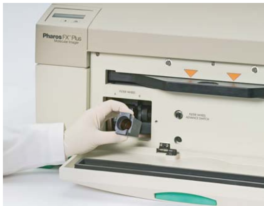
Fig. 4.6. Adding a new emission filter.
