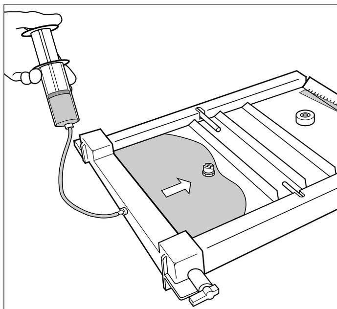
Fig. 4.7. Injecting gel solution into glass plate sandwich.
