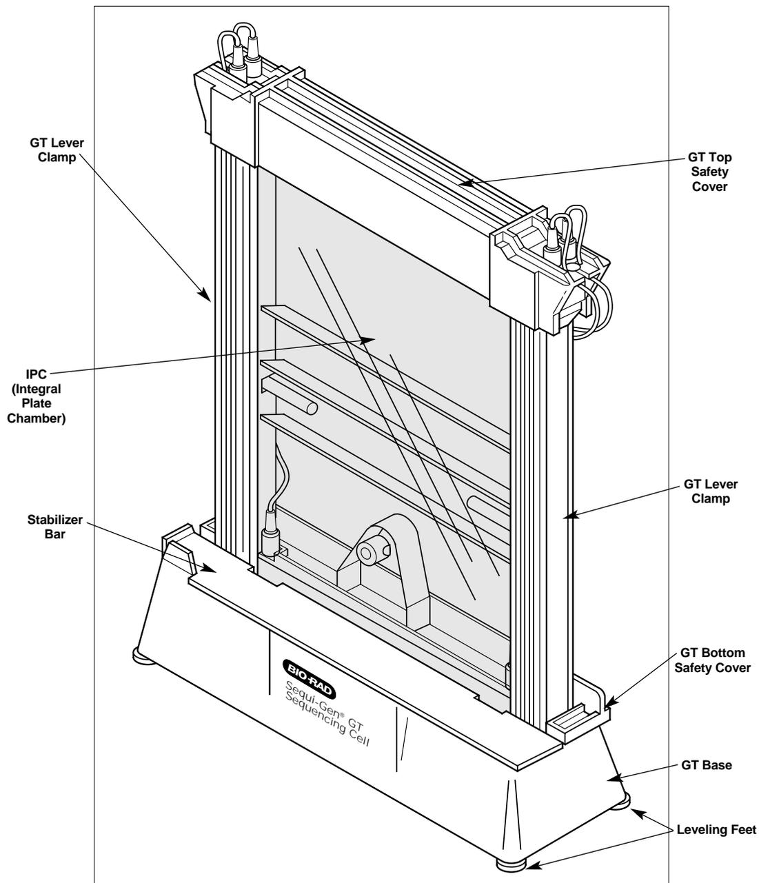
Fig. 2.2. Sequi-Gen GT nucleic acid electrophoresis cell.
