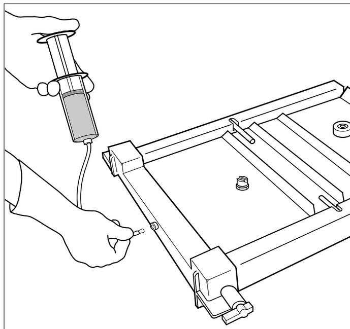
Fig. 4.6. Inserting syringe tubing into precision caster base.
