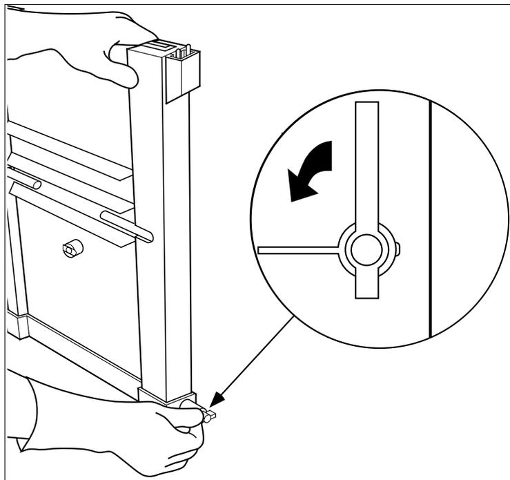
**Fig. 4.4. Attaching precision caster base to IPC assembly.**
