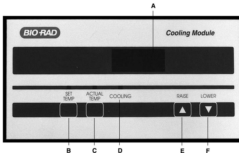
**Fig. 3. Control panel of Cooling Module.** A. Digital display (3 numerical places plus decimal point). B. Temperature set button and indicator light C. Actual temperature button and indicator light. D. Compressor running light. E. Raise button. F. Lower button.
