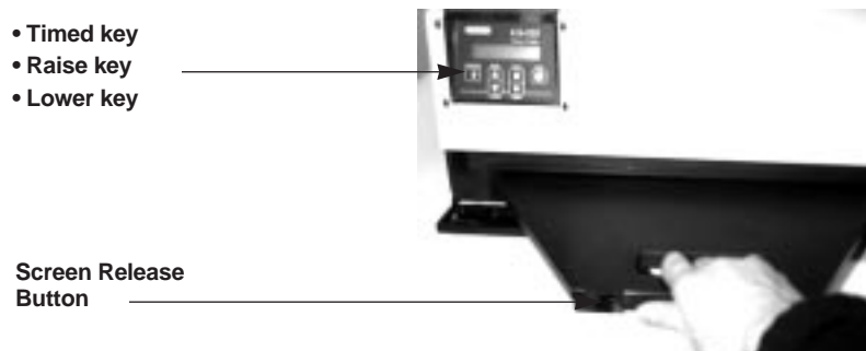
Fig. 4.2. Insertion of large format Imaging Screen into GS-525 Screen Eraser.
