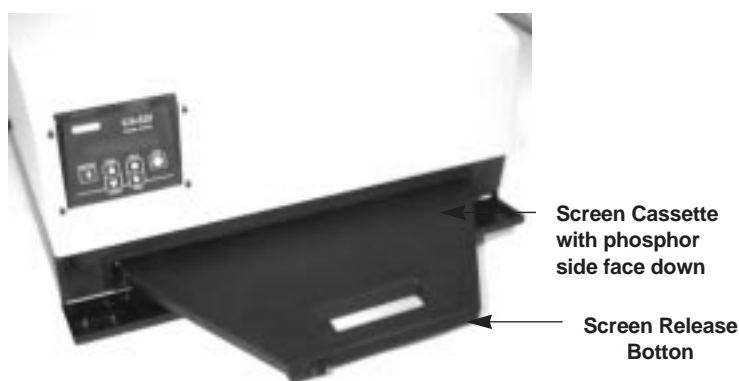
Fig. 4.5. Insertion of small Imaging Screen into the GS-505 Loading Dock.
