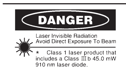
Fig. 1.4. Laser warning label visible when top cover is removed.
