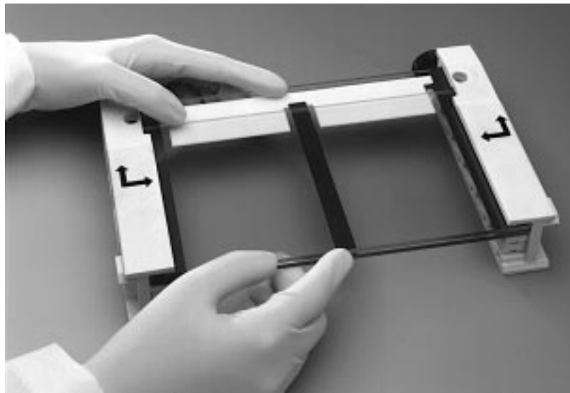
Fig. 6.4. Positioning the middle spacer in the sandwich assembly.
