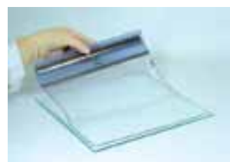
Using the gel clip to clamp onto a gel (PROTEAN Plus precast gel shown).
