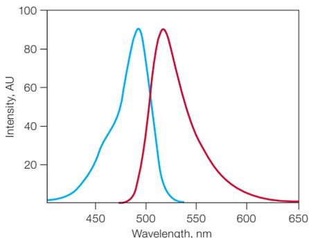
**Fig. 1. CFDA-SE excitation/emission is 492/517 nm in 0.1 M NaOH.** Excitation wavelength (—); emission wavelength (—). AU, absorbance unit.
