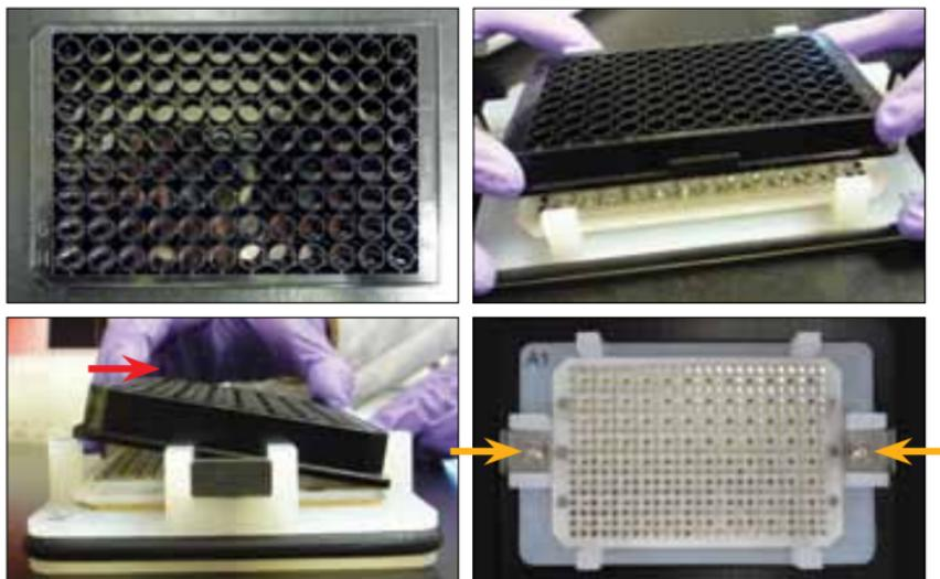
**Fig. 1. Setting up a new handheld magnetic washer.** The red arrow indicates the direction in which the assay plate is inserted. The yellow arrows indicate the direction in which the clips are pushed to secure the plate.
