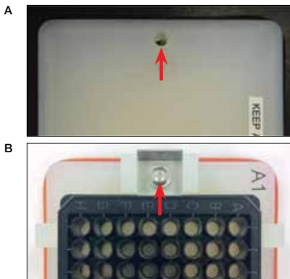
**Fig. 2. Adjusting clip height and tension. A,** Clip height adjustment. **B,** Clip tension adjustment. Red arrows indicate screw location.
