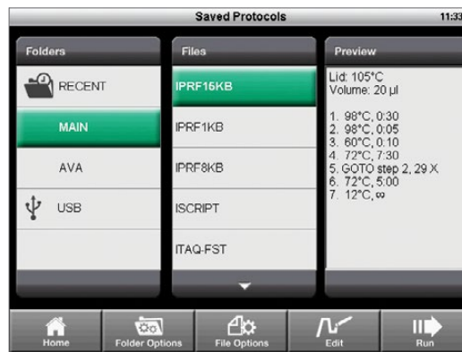
Fig. 6. Saved Protocols screen showing the preinstalled library of standard protocols in the MAIN folder.
