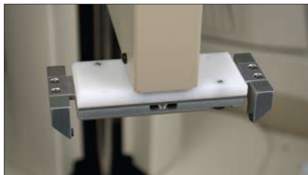
Fig. 4. Metal plate on the grippers.
