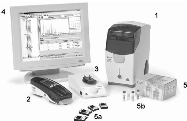
**The Experion system includes the following components:** 1) automated electrophoresis station, 2) priming station, 3) vortex station used for nucleic acid analysis only, 4) system operation and data analysis tools, and 5) analysis kits, which include the (a) chips and (b) reagents for protein (Pro260 kit), standard-sensitivity RNA (StdSens kit), high-sensitivity RNA (HighSens kit), and DNA (DNA 1K and 12K kits) analyses.
