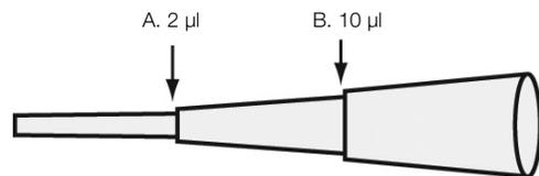
Fig. 1. Micropipet tip used for reproducible sampling of beads.
