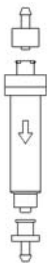
Fig. 3. Cartridge and fittings. Luer fittings and column: a cartridge should be mounted vertically with the arrow on the cartridge pointing downward.
