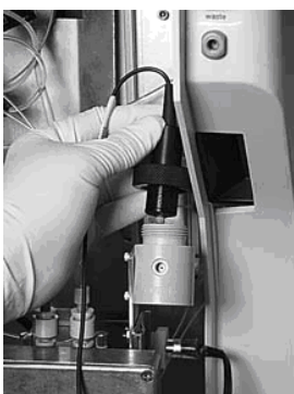
Installing flow cell
