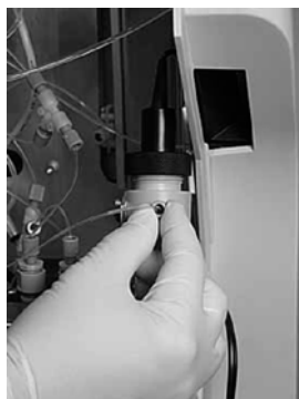
Connecting the tubing
