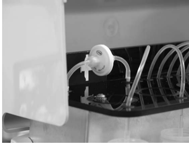
Location of the inline filter under the instrument top cover
