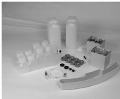
Fig. 1. Accessories for the Profinia instrument. Items shown include waste and diluent bottles (top), bottle starter pack (left), sample cooling device (right), cleaning tray (bottom), sample loop (bottom left), 15 ml and 50 ml sample lids and buffer bottle lids (middle).
