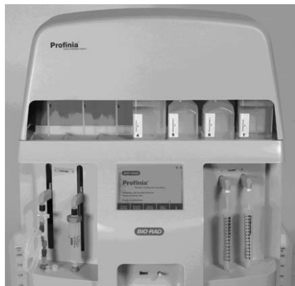
Fig. 6. Desalting sample loop and fittings.
