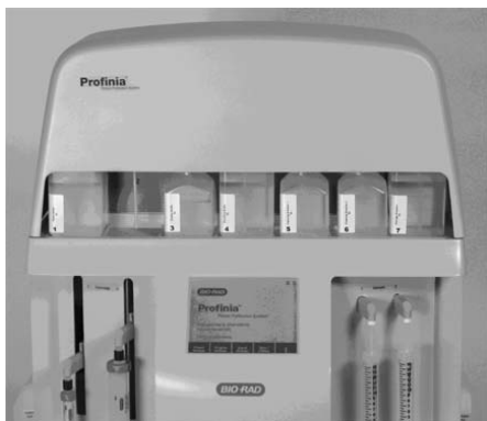
Fig. 4. Placement and positioning of GST buffers.
