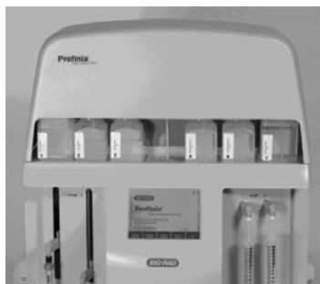
Fig. 3. Placement and positioning of denaturing IMAC buffers.
