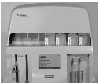
Fig. 5. Desalting and cartridge cleaning buffer bottle positioning.
