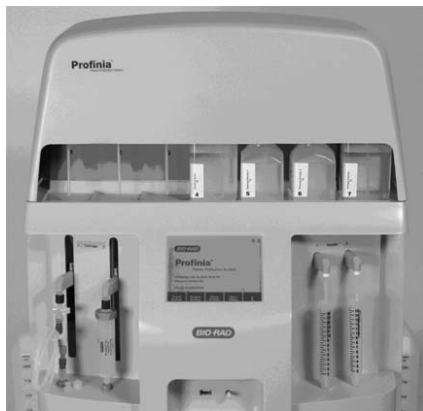
Fig. 6. Desalting sample loop and fittings.
