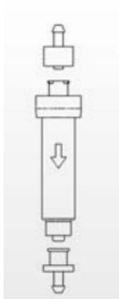
**Fig. 1. Luer fittings and column:** a cartridge should be mounted vertically with the arrow on the cartridge pointing downward.
