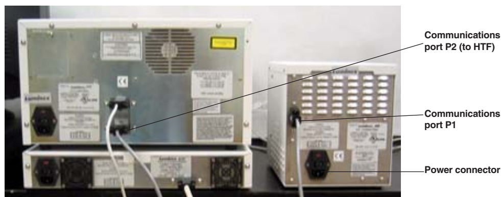
Fig. 7. HTF – rear panel view with connection to Bio-Plex 200 system.
