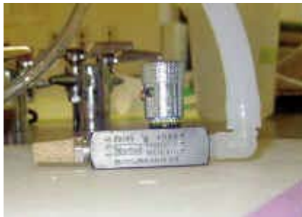
Fig. 23. Gold vacuum control valve.
