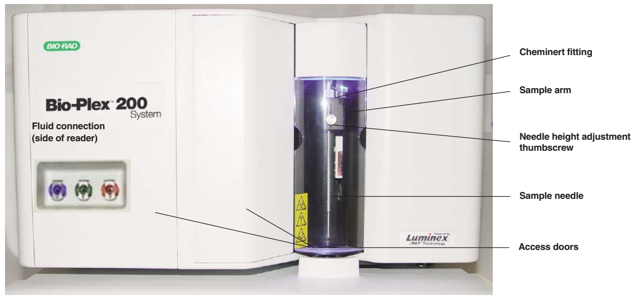
Fig. 1. Array reader – front and side panel features.
