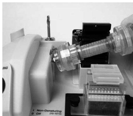
Fig. 13. Placing the focusing assembly onto the chassis.
