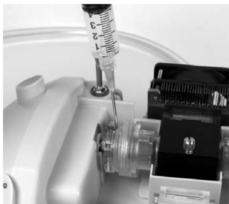
Fig. 15. Adding electrolyte to the anode assembly.
