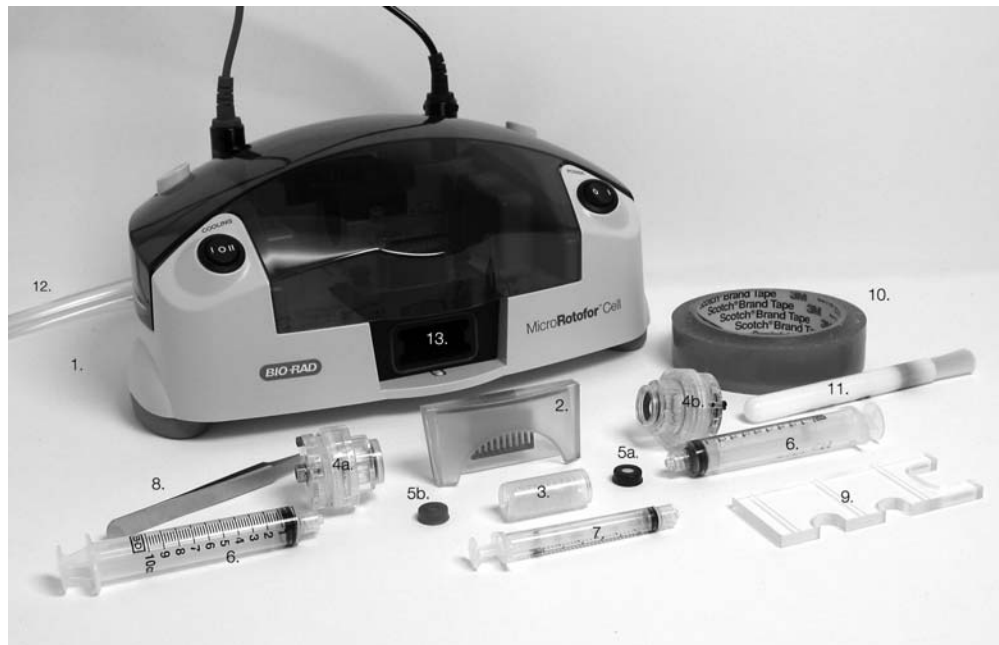
Fig. 1. MicroRotor components and accessories. MicroRotor chassis and lid (1), harvesting tray (2), focusing chamber (3), cathode assembly (4a), anode assembly (4b), cathode membrane, (5a), anode membrane, (5b), 10 ml syringes (6), 3 ml syringe (7), forceps (8), assembly tool (9), sealing tape (10), cleaning brush (11), vacuum hose (12), vacuum chamber (13).
