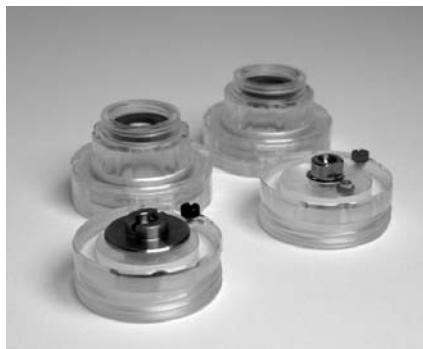
Fig. 4. Electrode assemblies. Left, components of the cathode assembly (black button); right, anode assembly (red button). The threaded sleeves are shown attached to the electrolyte components.
