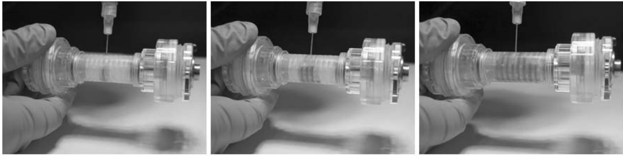
Fig. 12. Loading sample into the focusing chamber.
