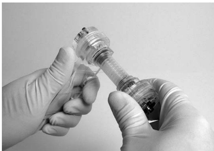
Fig. 19. Using the assembly tool to remove the anode assembly from the focusing assembly.
