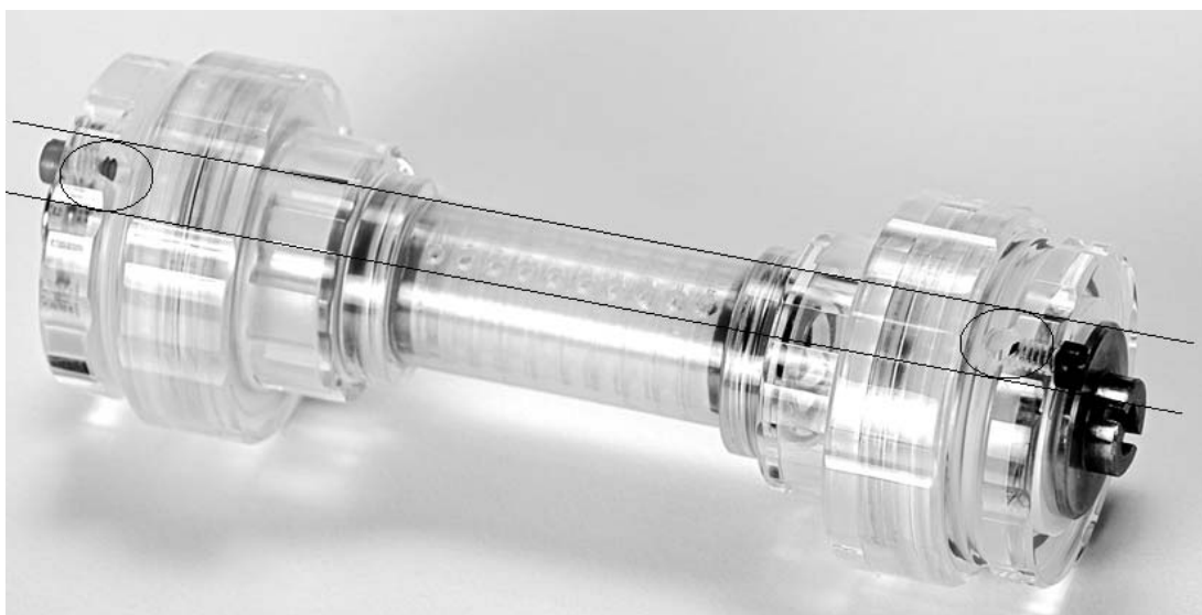
Fig. 9. Alignment of the sample loading ports with the vents on the anode (left) and cathode (right) assemblies.
