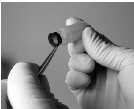
Fig. 6. Inserting an anion exchange membrane into the focusing chamber.
