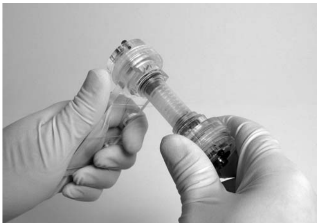
Fig. 8. Using the assembly tool to securely attach an electrode assembly onto the focusing chamber.
