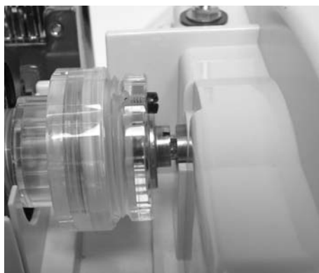
Fig. 14. Fitting the cathode assembly into the notch of the chassis.
