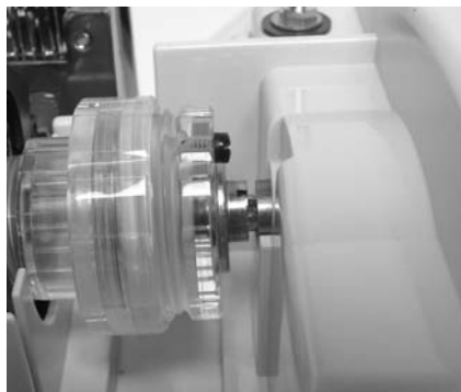
Fig. 8. Fitting the cathode assembly into the cathode of the chassis.
