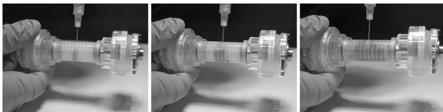
Fig. 6. Loading sample into the focusing chamber.
