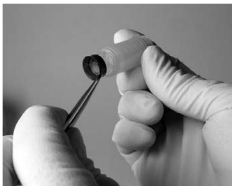
Fig. 2. Inserting an anion exchange membrane into the focusing chamber.
