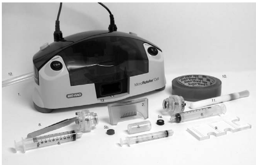
Fig. 1. MicroRotor components and accessories. MicroRotor chassis and lid (1), harvesting tray (2), focusing chamber (3), anode assembly (4a), cathode assembly (4b), cathode membrane, (5a), anode membrane, (5b), 10 ml syringes (6), 3 ml syringe (7), forceps (8), assembly tool (9), sealing tape (10), cleaning brush (11), vacuum hose (12), vacuum chamber (13).
