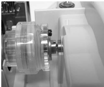
**Fig. 8. Fitting the cathode assembly into the cathode of the chassis.**
