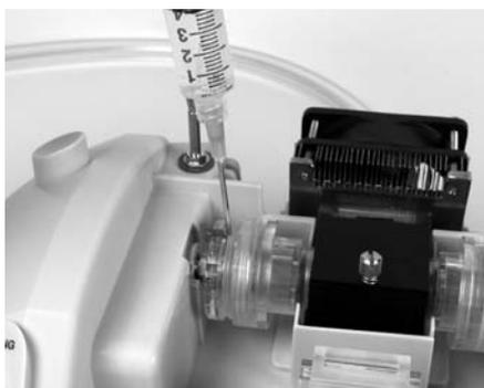
**Fig. 9. Adding electrolyte to the anode assembly.**
