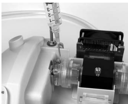
Fig. 9. Adding electrolyte to the anode assembly.
