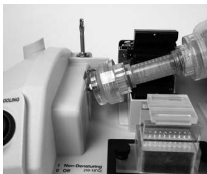
Fig. 7. Placing the focusing assembly onto the anode of the chassis.
