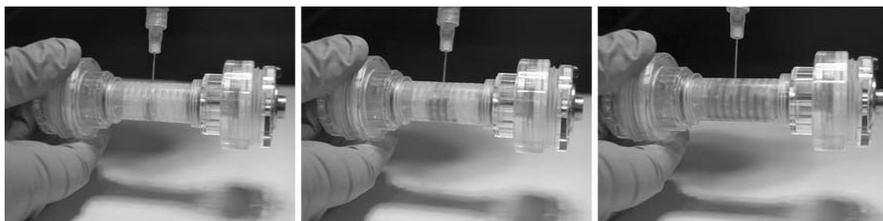
**Fig. 6. Loading sample into the focusing chamber.**
