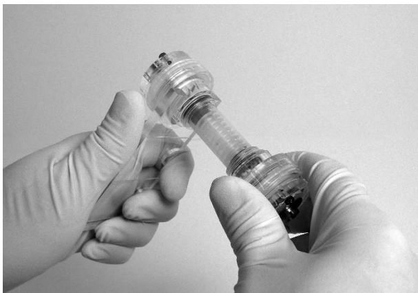
Fig. 14. Using the assembly tool to remove the anode assembly from the focusing assembly.
