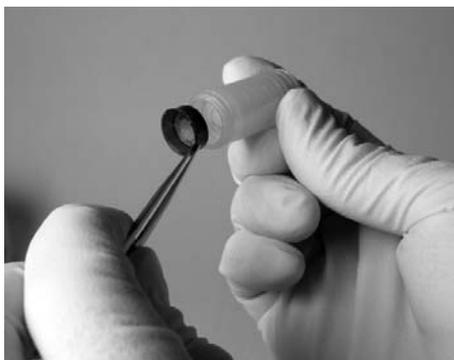
**Fig. 2. Inserting an anion exchange membrane into the focusing chamber.**
