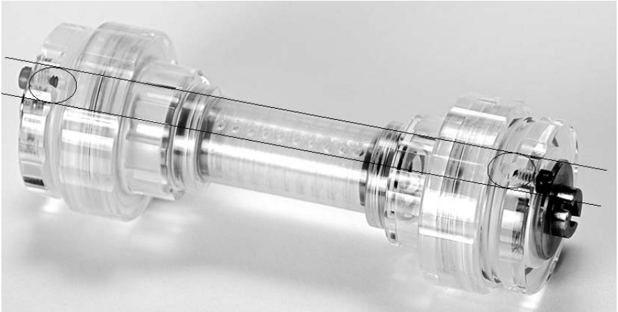
Fig. 3. Alignment of the sample loading ports with the vents on the anode (left) and cathode (right) assemblies.
