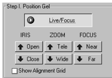
Fig. A-3. Newer Gel Doc EQs feature camera control buttons in the acquisition window.
