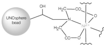
**Fig. 1. Partial structure of Profinity Ni-charged IMAC resin.**
